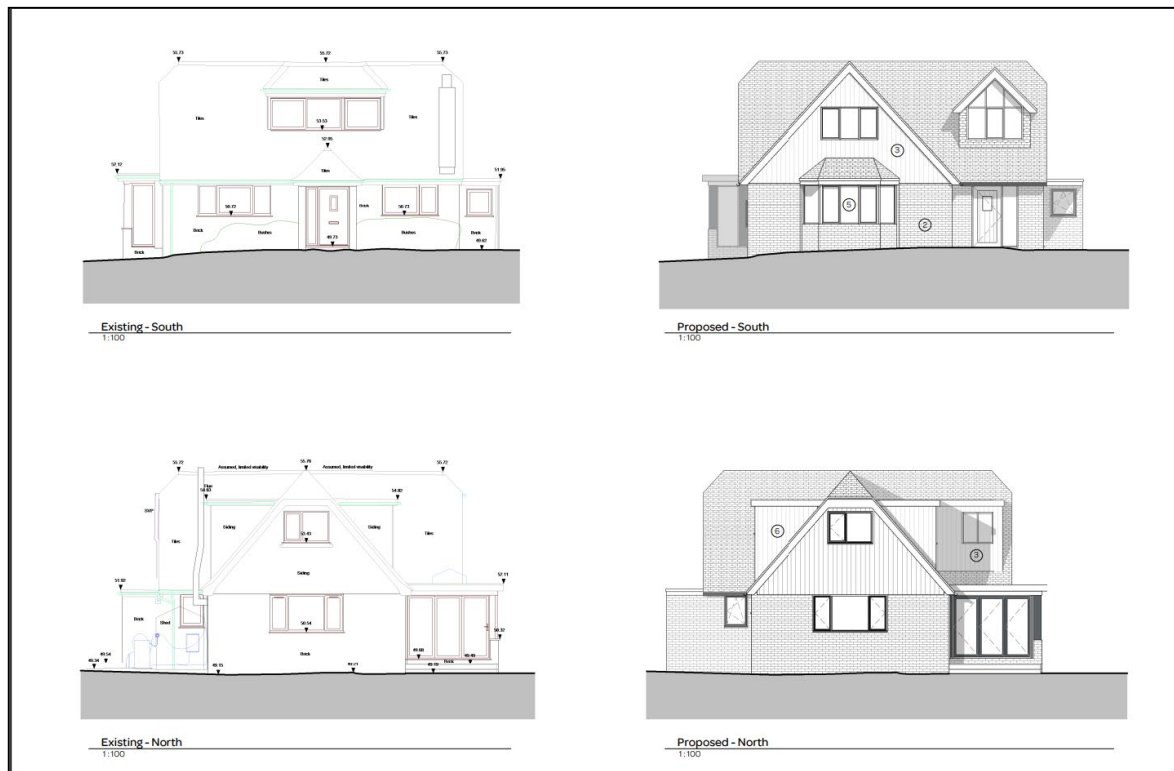
Figure 2: Existing and proposed South & North Elevations
