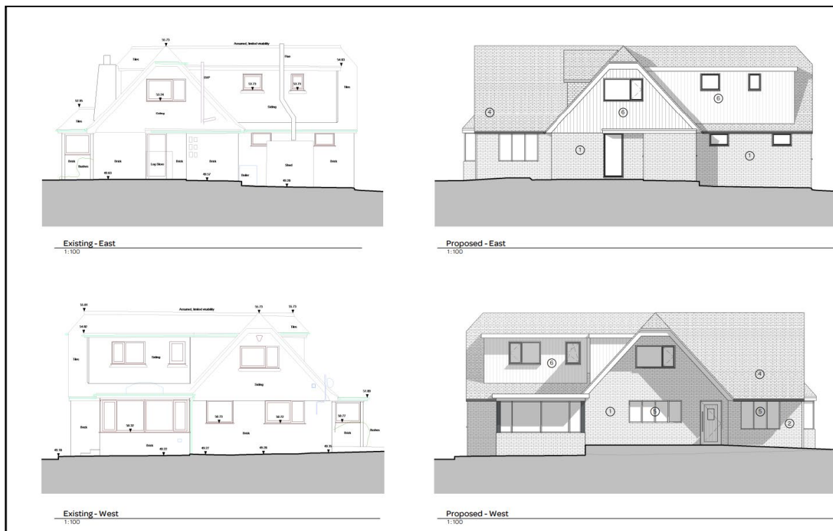
Figure 3: Existing and proposed East & West Elevations
