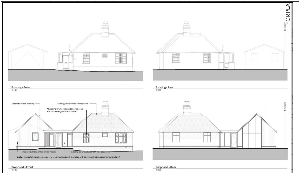
Figure 4: Existing and proposed front & rear elevations
